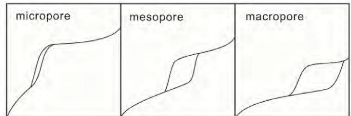
Fig. 11—Effect of pore size to adsorption isotherm curve in shale.
